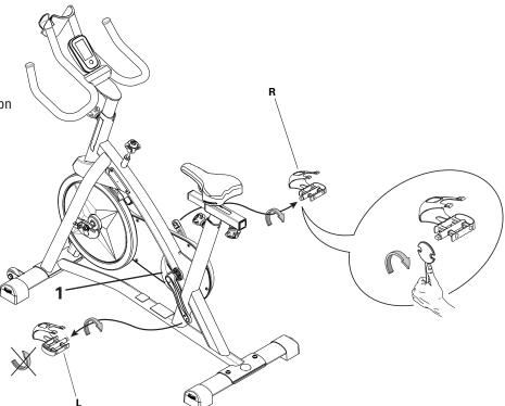
**3.** Carefully remove the Chain Guard Center from the Chain Guard Cover, and and set it safely aside for reassembly.
