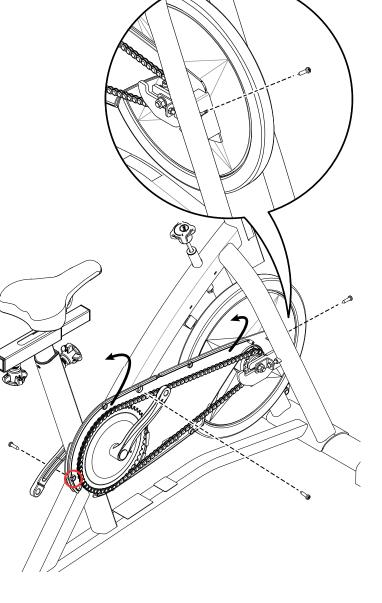
**14.** Mark the position of the Flywheel Retainer Clips (A) on the flywheel brackets (B) on the Frame. Record the number of threads showing on the Hex Head Bolt (C) that attaches each Flywheel Retainer Clip to the Frame.
