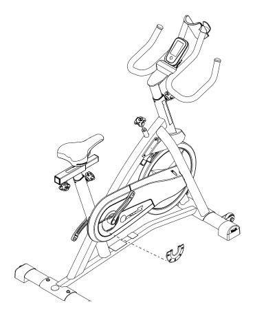
**4.** Loosen and remove the hardware that attaches the Chain Guard Cover to the Chain Guard Inside. Carefully remove the Chain Guard Cover and discard it.
