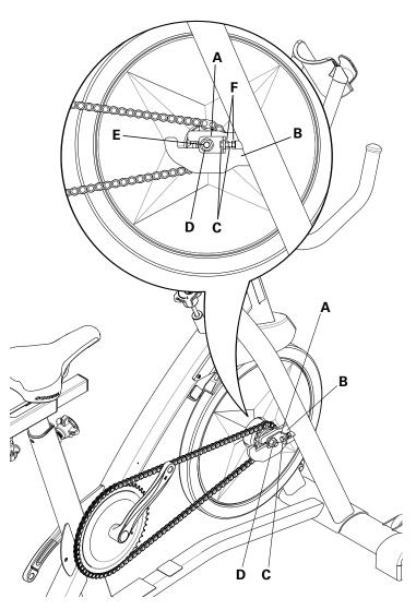
**10.** To loosen the Flywheel hardware, use a 15 mm crescent wrench to hold the Axle Nut (D) on one side steady and loosen the Axle Nut on the opposite side with a 15 mm socket and wrench. Remove the Axle Nut from the Flywheel axle (E). Set the hardware safely aside for reassembly.
