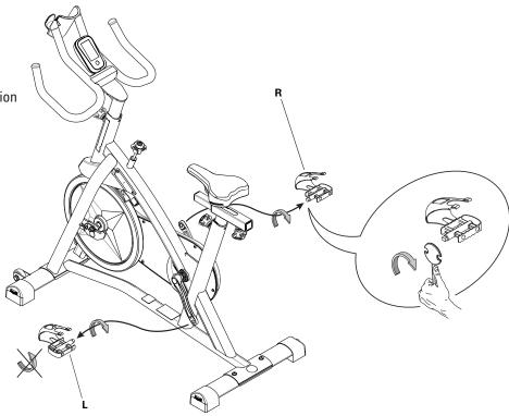
2. Install the new Pedals. Carefully align the threads and hand tighten to prevent crossthreading. Then tighten fully with pedal wrench.
