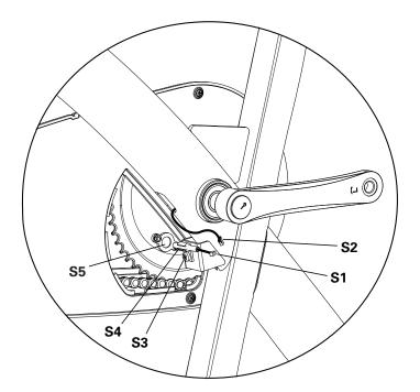
7. Loosen and remove the hardware that attaches the Chain Guard Inside to the Main Frame. Set the hardware safely aside.
