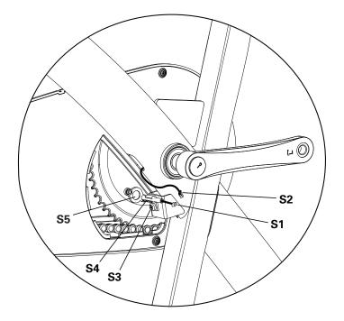
. Loosen and remove the hardware that attaches the Chain Guard Inside to the Main Frame. Set the hardware safely aside.
