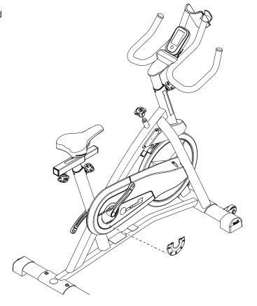
**4.** Loosen and remove the hardware that attaches the Chain Guard Cover to the Chain Guard Inside. Carefully remove the Chain Guard Cover and set it safely aside for reassembly.
