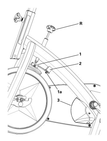
**8.** Carefully remove the Chain Guard Center from the Chain Guard Cover, and and set it safely aside for reassembly.
