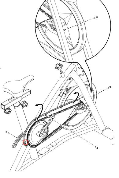
**9.** Mark the position of the Flywheel Retainer Clips (A) on the flywheel brackets (B) on the Frame. Record the number of threads showing on the Hex Head Bolt (C) that attaches each Flywheel Retainer Clip to the Frame.
