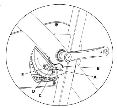
7. Loosen and remove the hardware that attaches the Chain Guard Inside to the Main Frame. Set the hardware safely aside.
