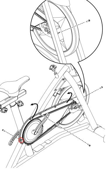
**9.** Mark the position of the Flywheel Retainer Clips (A) on the flywheel brackets (B) on the Frame. Record the number of threads showing on the Hex Head Bolt (C) that attaches each Flywheel Retainer Clip to the Frame.
