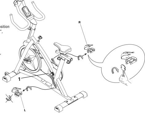
**3.** Carefully remove the Chain Guard Center from the Chain Guard Cover, and and set it safely aside for reassembly.
