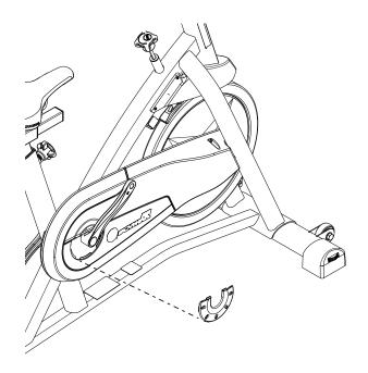
3. Remove the hardware that attaches the Chain Guard Cover to the Chain Guard Inside, and set it safely aside for reassembly. Carefully remove the Chain Guard Cover and set it safely aside for reassembly.
