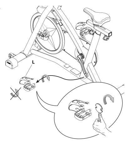
**2.** Using a flathead screwdriver, remove the threaded Cap (B) from the Crank Arm (A).
