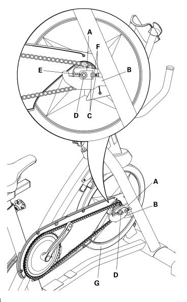
**5.** To loosen the Flywheel hardware, use a 15 mm crescent wrench to hold the Axle Nut (D) on one side steady and loosen the Axle Nut on the opposite side with a 15 mm socket and wrench. Remove the Axle Nuts from the Flywheel axle (E). Set the hardware safely aside for reassembly.
