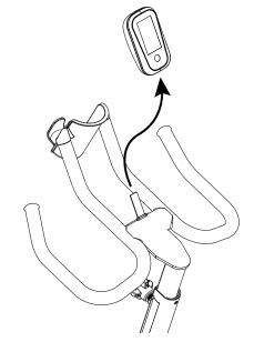
2. Loosen and remove the hardware that attaches the Water Bottle Holder, and set it safely aside for reassembly. Remove the Water Bottle Holder, and set it safely aside for reassembly.
