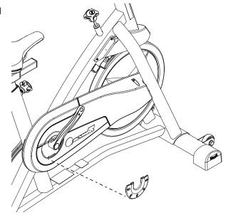
3. Remove the hardware that attaches the Chain Guard Cover to the Chain Guard Inside, and set it safely aside for reassembly. Carefully remove the Chain Guard Cover and set it safely aside for reassembly.
