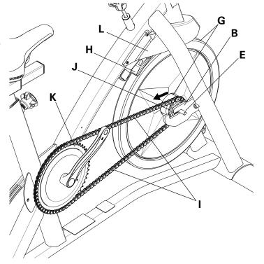
**14.** Using a flathead screwdriver, remove the threaded Cap (L) from the Sprocket Drive/Crank Arm assembly (K).
