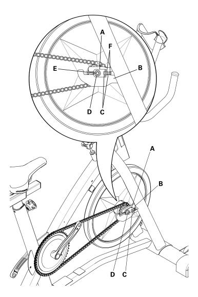
**15.** To loosen the Flywheel hardware, use a 15 mm crescent wrench to hold the Axle Nut (D) on one side steady and loosen the Axle Nut on the opposite side with a 15 mm socket and wrench. Remove the Axle Nuts from the Flywheel axle (E). Set the hardware safely aside for reassembly.
