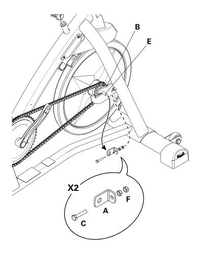
**12.** Carefully move the Flywheel (G) to the opening in the flywheel brackets (B). Carefully lift the Drive Chain (I) off the Flywheel sprockets (J) to the outside.
