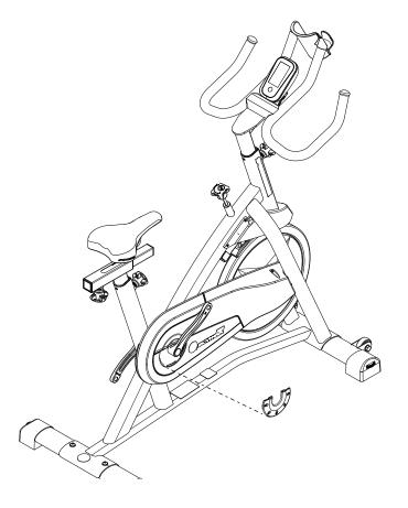
**4.** Loosen and remove the hardware that attaches the Chain Guard Cover to the Chain Guard Inside. Carefully remove the Chain Guard Cover and set it safely aside for reassembly.
