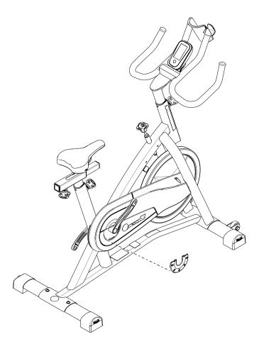
**9.** Loosen and remove the hardware that attaches the Chain Guard Cover to the Chain Guard Inside. Carefully remove the Chain Guard Cover and set it safely aside for reassembly.
