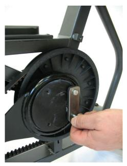
12. Remove the hardware from the Removal Plate using the 10 mm socket and wrench.
