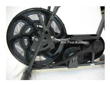
8. Slide the Arm Pivot Assembly off of the machine.
