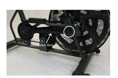
9. Using a 15 mm wrench, remove the Eye Bolt Securing Nut from both sides of the machine.
