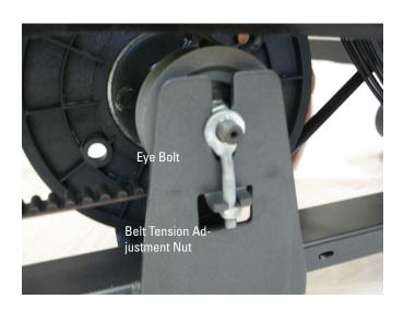
30. Using a 15 mm wrench, attach the Securing Nuts for the Eye Bolt on both sides of the machine.
