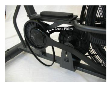
14. Remove the Crank Belt by sliding it forward off of the Connector Arm.
