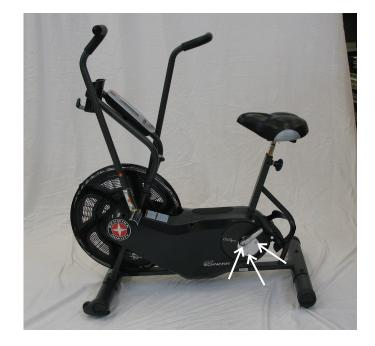
2. Using a #2 Phillips screwdriver, remove the indicated screws from the Shrouds.
