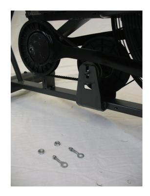
12. Gradually work the Pulley Assembly out of the Bracket.
