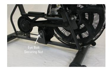
10. Using a 10 mm wrench, loosen the Belt Tension Adjustment Nut and remove the Eye Bolt.
