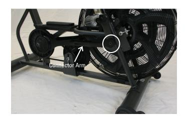
9. Using a 15 mm wrench, remove the Eye Bolt Securing Nut from both sides of the machine.
