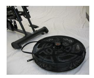
24. Route the Fan Belt into the new Fan Assembly, and over onto the Fan Assembly Pulley.
