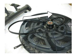
25. Insert the new Fan Assembly with Fan Belt into the Frame Assembly.
