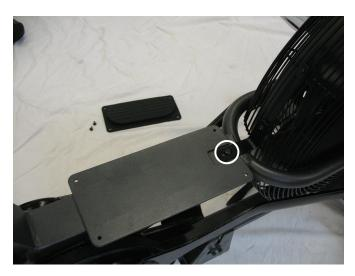
18. Using a #2 Phillips screwdriver, remove the 2 indicated screws from each side of the Fan Assembly.
