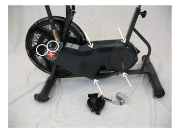
3. Remove the Shroud and Crank Cover.
