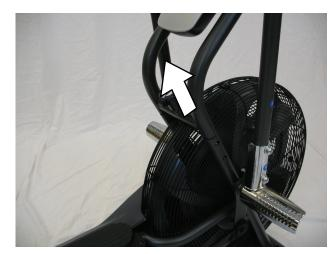
4. Disconnect the Cables and place the Console Support Bar Assembly on the floor safely out of the work area.
