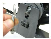
29. Gradually tighten the Belt Tension Adjustment Nuts by a full turn, alternating between each side. Continue until the Crank Belt (700-800N) and the Drive Belt (400N) can barely be pushed at their mid-point.
