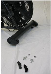
23. Pulling from the front of the machine, remove the Fan Assembly from the Frame Assembly.
