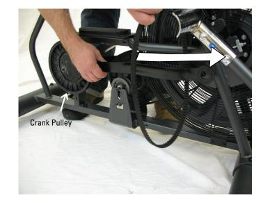
15. Route the new Crank Belt over the Connector Arm and onto the Crank Pulley.
