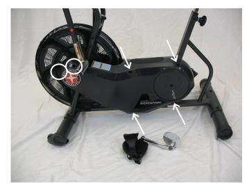
3. Remove the Shroud and Crank Cover.
