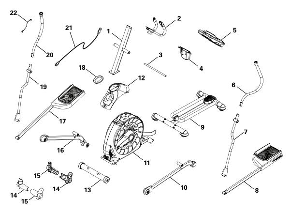
A decal has been applied to all right ("  ${f R}$  ") and left ("  ${f L}$  ") parts to assist with assembly.
