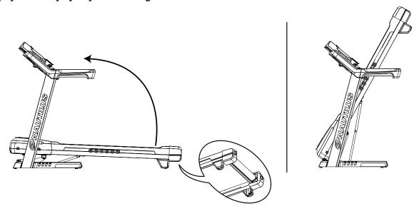
6. Make sure that the locking mechanism is engaged. Carefully pull back on the walking deck and make sure that it does not move. When you do this, keep clear of movement path in case the treadmill lock is not engaged.
