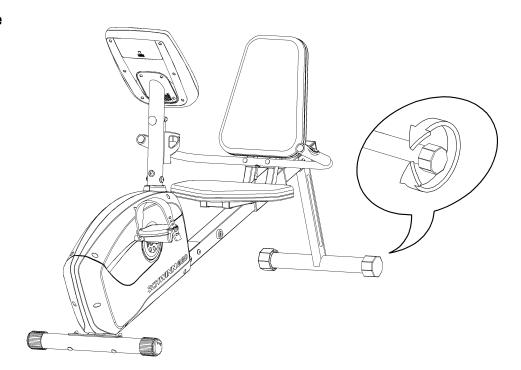
The levelers are the polygonal end caps on the Rear Stabilizer. Turn the end cap to adjust the level. Make sure the bike is level and stable before you exercise.
