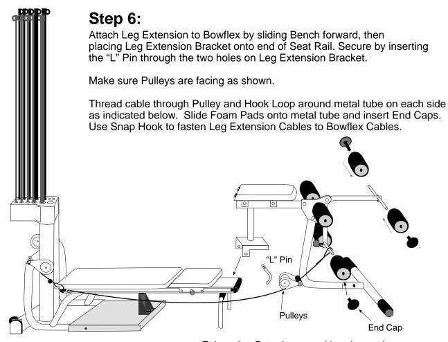
To leave Leg Extension on machine when not in use, unhook Leg Extension Cables from Bowflex Cables.
