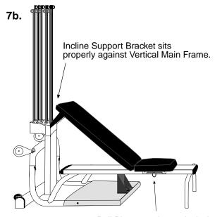
Pull Pin out and turn clockwise. one quarter turn to lock Seat into position.
