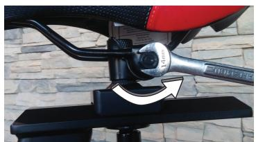
**3.** Place the new Seat onto the Post. Tighten both nuts (B) on the Seat bracket (A) to hold the Seat in position.
